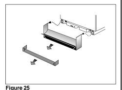
After installation, water and electrical lines are connected and the unit leveled, assemble the base part (see below).
